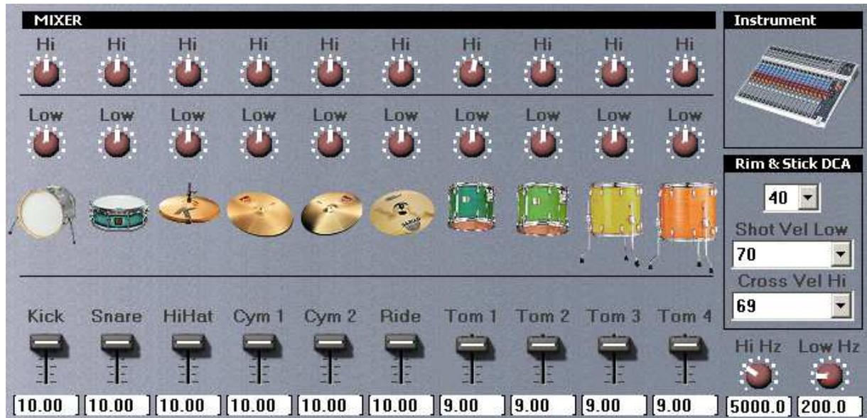
This slot-type gives you a virtual mixer. Associated drum-tracks get bundled with drums and can be adjusted for volume and with the 2-band-equalizers fine tuned. Finally all the single drums of the drum sets/programs can be fine tuned to each other. The Equalizer gives you two shelving filters to adjust the high and low frequencies (Hi Hz, Low Hz). With the Hi and low controllers you can adjust the intensity of the sound changes.
